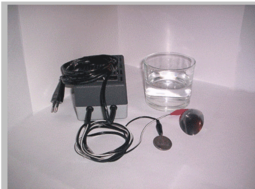
A simple home made Electrolysis machine. It consists in an AC adapter having alligator clips on 6V cable ends. One old spoon has been attached to the positive alligator clip, while the coin is attached on the negative one.
